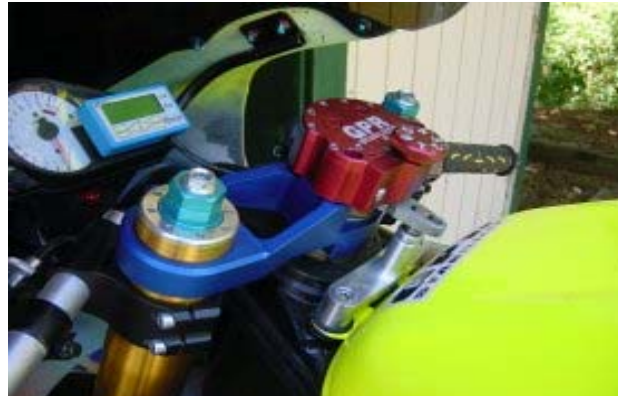
Typical application of a GPR rotary steering stabilizer on a sport bike
